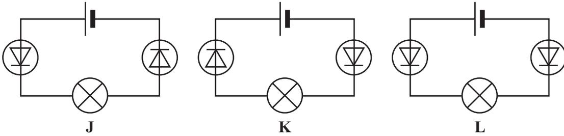
In which **one** of the circuits, **J**, **K** or **L**, would the filament lamp be on?
